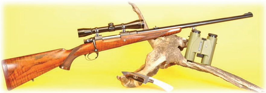
[The author's beautiful 9.3X62 built on a Brno ZG47 action - Pierre van der Walt]
